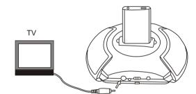
(5) Connect with TV by RCA cable for video output
